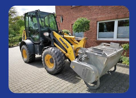
To be connected to a hydraulic quick change device or 3rd control circuit
